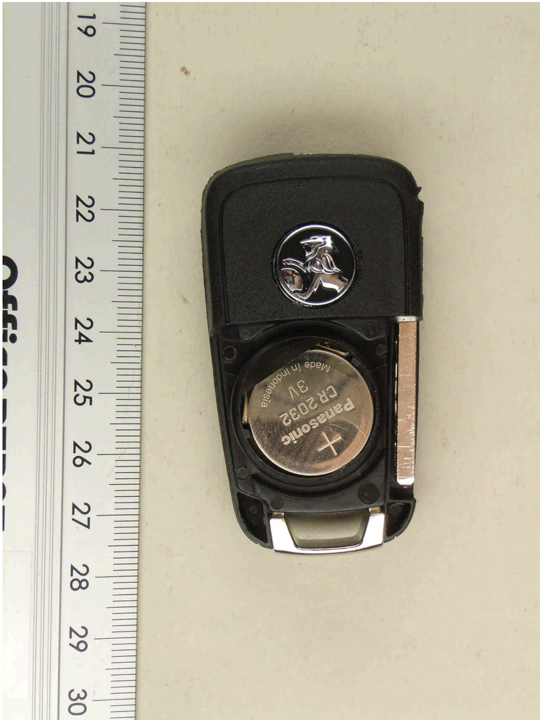
101794_23.jpg Global A Flap Key , Battery cover removed
