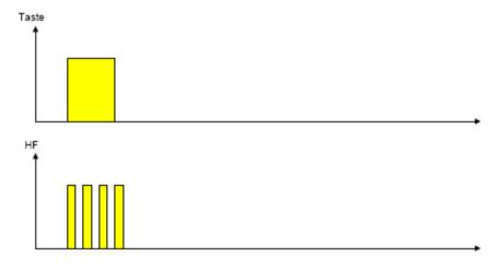
A short valid button pressing results a sending of the minimum number of the RF telegrams, as showed on the diagram.
