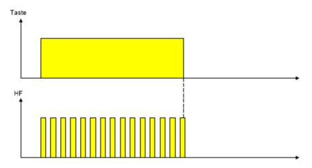
If the duration of the button pressing extents the time required for transmitting the minimum amount of RF telegrams, additional telegrams will be sent until the button is released or a timeout of 25s is reached. This timeout function prevents the unintended transmission over the extended time periods in case of a button was fixed.
