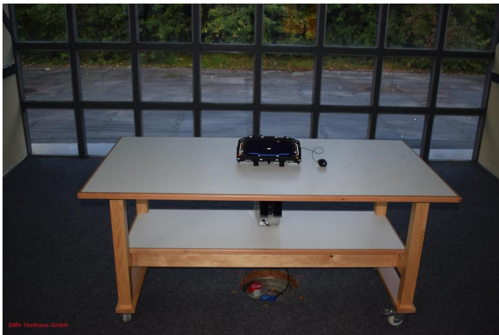
Picture 4: OATS, test setup final radiated emission test (front view)
