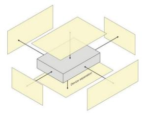
Figure 1: Test position for a generic device
