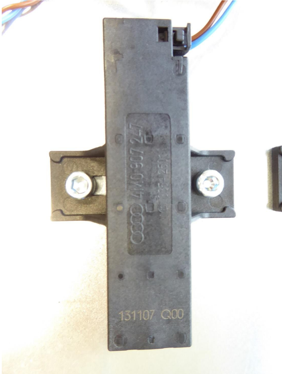
154295_8.JPG: LF antenna type 1
