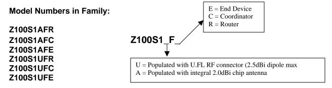
Aerocomm's Z100S1 family of 2.4Ghz Zigbee transceivers is made up of 6 different model numbers. The hardware platform for the Z100S1 family has the option for either an integral chip antenna or a U.FL RF connector. Three different types of firmware options are also available. Either Coordinator, Router, or End Device firmware is programmed at the factory.
