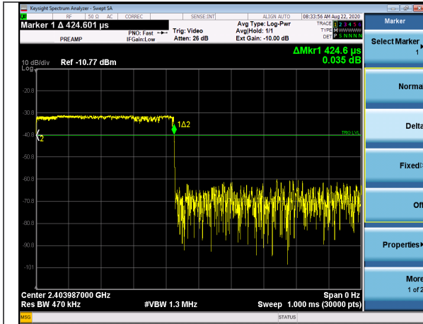
Low Channel Occupancy Time
