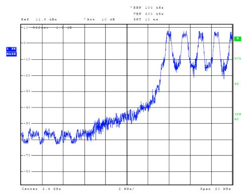
Figure Ten of Antenna Port Conducted Emissions (Low Band Edge)
