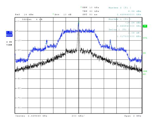
Figure Eight of Antenna Port Conducted Emissions (Occupied Bandwidth 2435)
