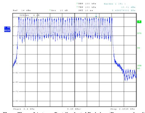
Figure Three of Antenna Port Conducted Emissions (Frequency band)
