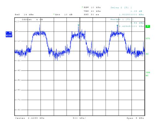
**Figure Four of Antenna Port Conducted Emissions (Channel Separation)**
