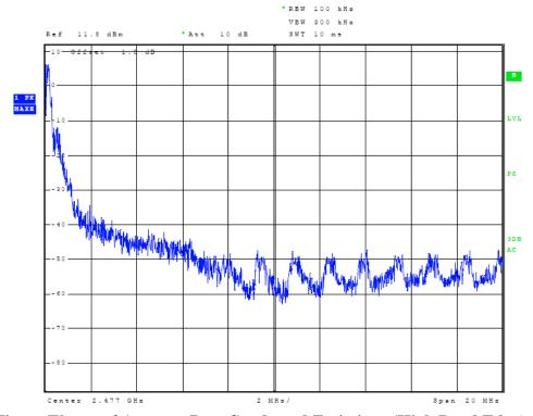
Figure Eleven of Antenna Port Conducted Emissions (High Band Edge)
