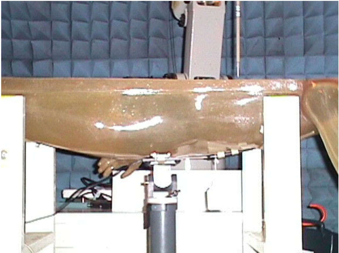
< Waist with the Nearson, S181FL-5-RMM-2450S ¼ wave dipole antenna, 10mW unit – Overview >
