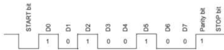
Figure 4: Even Parity Bit
