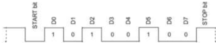
Figure 3: Asynchronous Mode Signal
