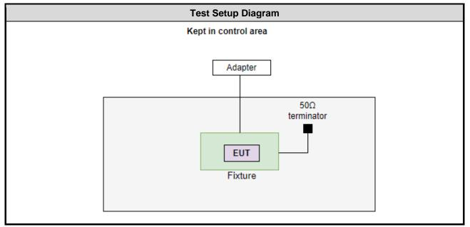
Note: The PC and RS232 cable are disconnected from EUT and removed from test table when EUT is set to transmit continuously.
