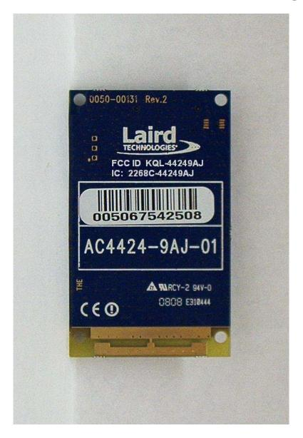
The FCC & IC identification will be permanently screen printed on the back of the board above the serial number in white lettering as shown above.
