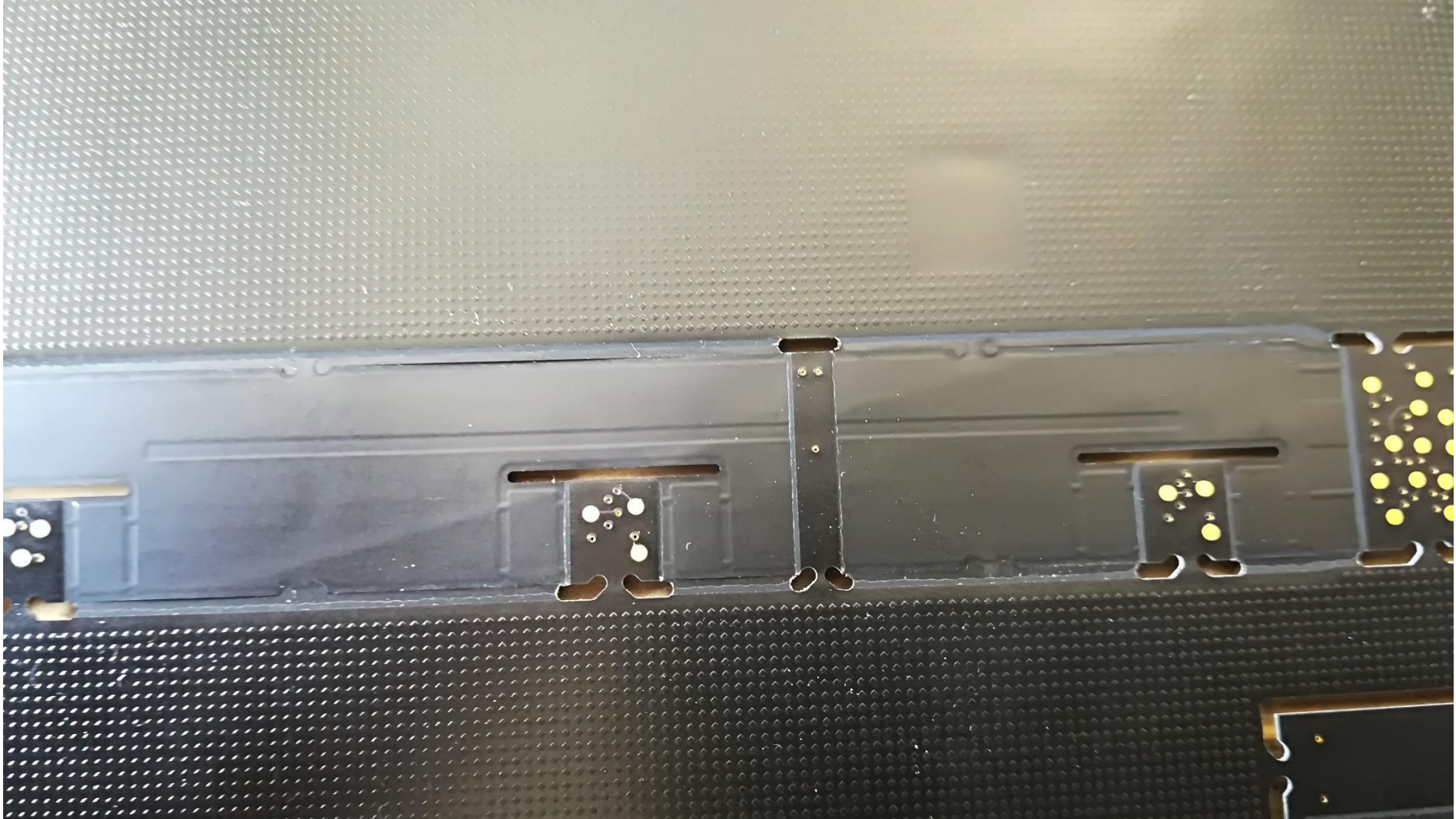
Photo 5. RMP400 Flexi-Rigid PCB Slot Antenna (bottom side view)
