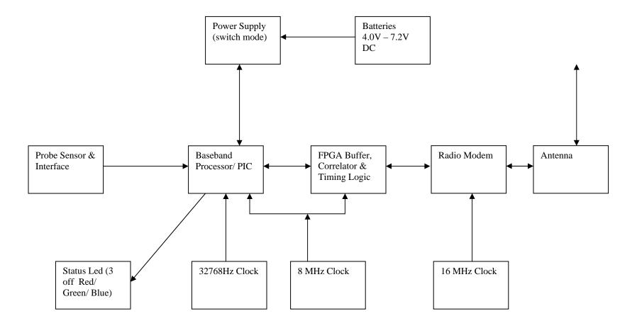
Fig 2 RMI Functional block diagram
