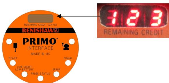
4. Low battery/credit output from the Interface, which can be connected to the machine control. When credit is running low, an alarm will be sent to the control.
