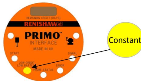
3. Interface digital display (123 days remaining shown). When the remaining credit display reads 0 days then the Primo System will stop working and new credit will need to be loaded into the system.
