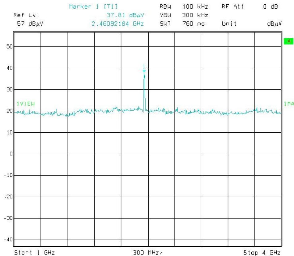
Transceiver A – Channel 11      Horizontal Polarisation
