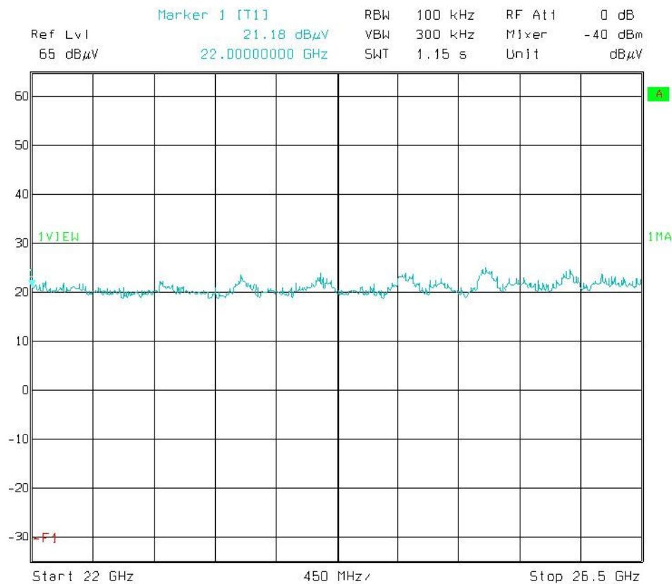
Transceiver A – Channel 11      Horizontal Polarisation
