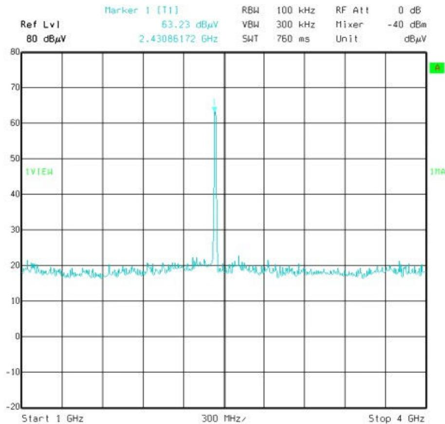
Transceiver A – Channel 6      Vertical Polarisation
