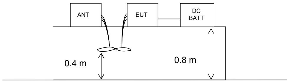
The EUT and peripheral equipment were placed on a non-conducting table, 0.8 m above a ground plane. Excess cables were bundled and kept at a distance of 0.4 m from the ground plane. Each piece of equipment was positioned 0.1 m apart, with the rear of the equipment positioned flush with the edge of the non-conducting table. To identify frequencies of interest the measuring antenna was moved over the surfaces of the EUT and peripheral equipment.
