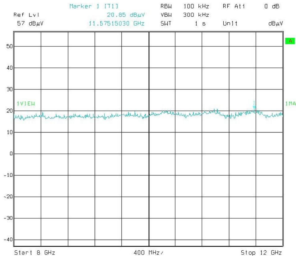
Transceiver A – Channel 11      Vertical Polarisation
