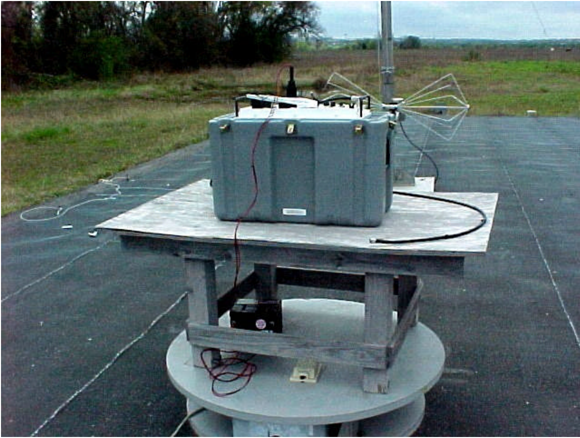
Photo 2. The REM on turntable at OATS.
