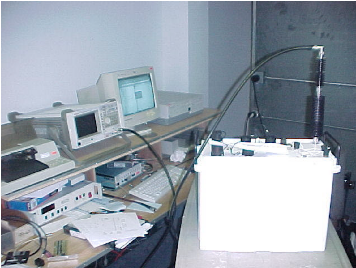
Photo 1. spurious emissions measurement. Attenuators totaling 70 dB reduce output power to a level appropriate for spectrum analyzer measurement without front-end compression.
