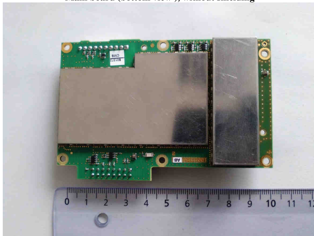
Main board (bottom view) with shielding
