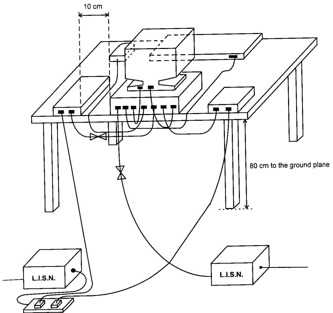
**5.4. TEST RESULT OF AC POWERLINE CONDUCTED EMISSION**
