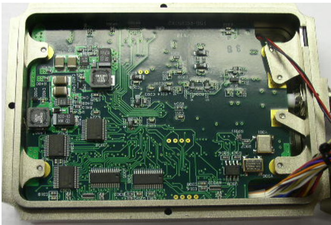
Figure 8 – Interior top half (solder side) SDI board assembly
