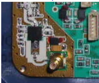
Figure 5 – Interior bottom half (component side) Tx Board assembly
