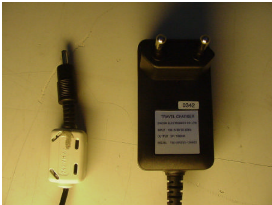
Picture 3 : EUT B, Cincon charger (with ferrit)
