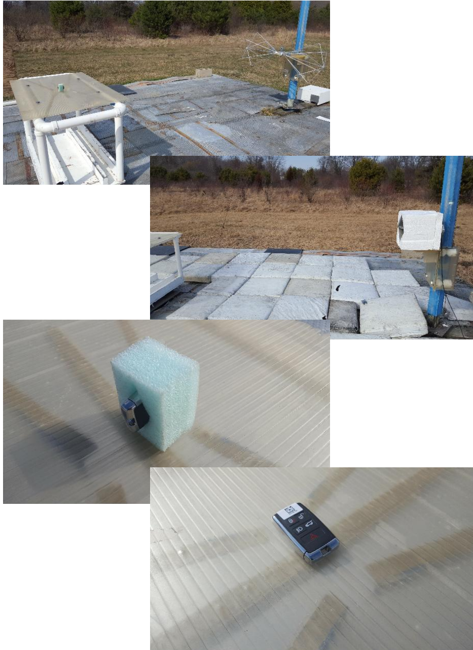
Figure 4: Radiated Emissions Test Setup Photograph(s).
