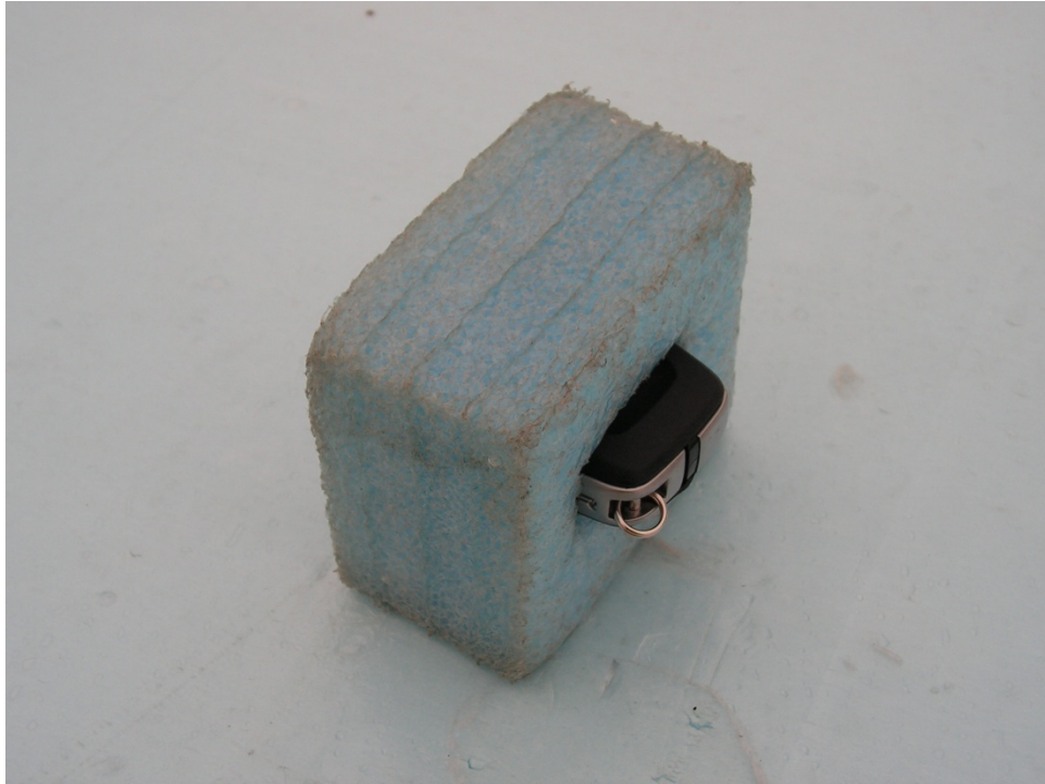
Photograph 6.6. Close-up of DUT on OATS with drawers closed (one of three axes tested)
