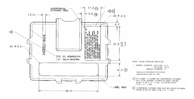
The top side of the module has OEM and Module Manufacturer information molded into the housing.
