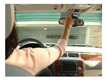
To program another rolling code device such as an additional garage door opener, a security device, or home lighting, repeat steps 1-4 substituting a different function button in Step 3 than what you used for the garage door opener. For example, you could assign the left-most button to the garage door, the center button to a security device, and the right-most button to another garage door opener.
