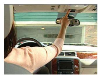
Immediately (within 1 second) release the button once the garage door moves. During this time the selected button indicator light will blink slowly. Do not release the button until you see the garage door move. Most garage doors open quickly. You may need to hold the button from 5-55 seconds before observing movement of the garage door.
