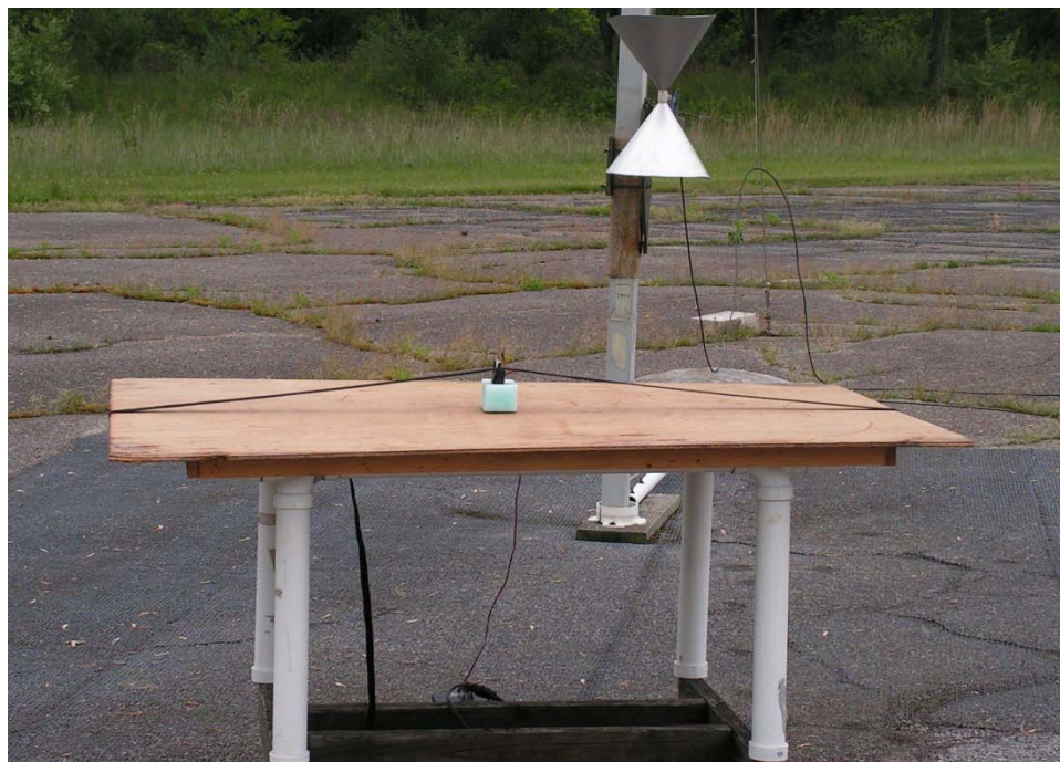
Photograph 6.5. DUT on OATS (one of three axes tested)
