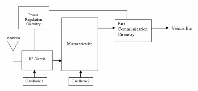
oscillator circuit 1 is at 9.5094 MHz and oscillator circuit 2 is at 8.00 MHz.
