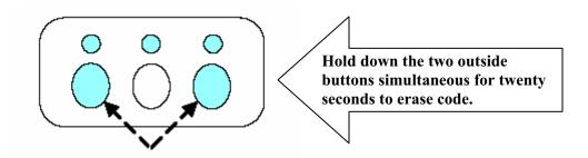
2. Once the indicator lights begin to blink, RELEASE your fingers from the buttons. The codes for all buttons (fixed and rolling code) are erased.
