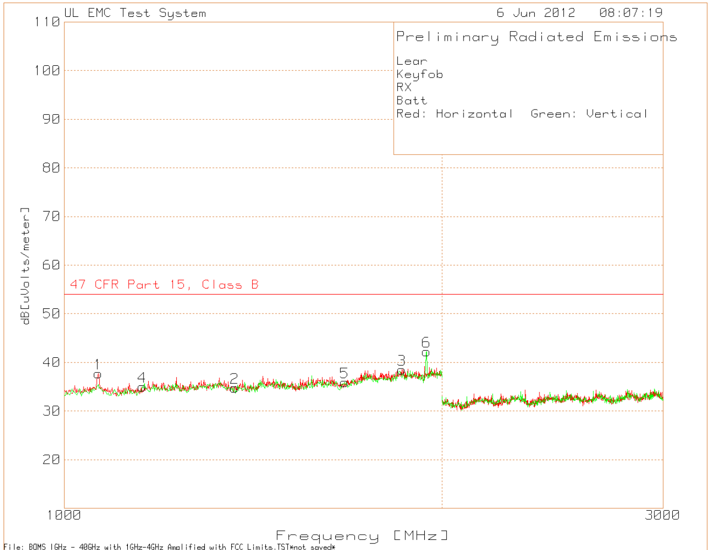
Figure 16 Radiated Emissions Graph RX 1-3 GHz Z-Axis
