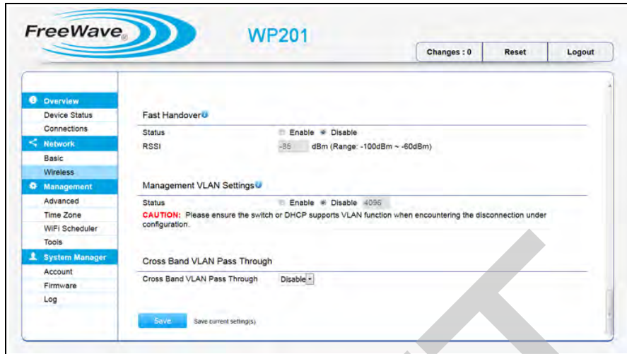
Figure 53: Wireless window - Fast Handover, Management VLAN Settings, and Cross Band VLAN Pass Through areas
