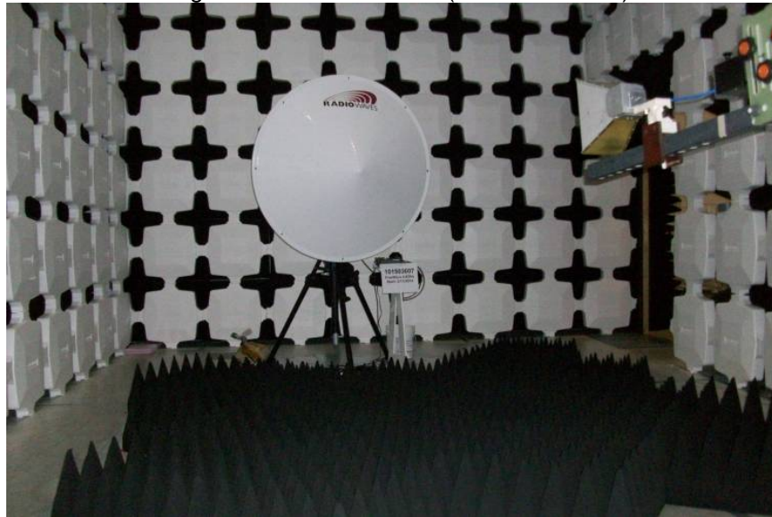
Ridge-Guide Horn Antenna (1GHz to 18GHz)
