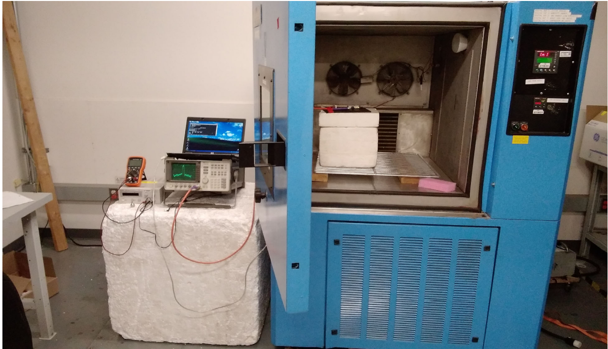
Test Configuration Photograph #5 (Frequency Stability)
