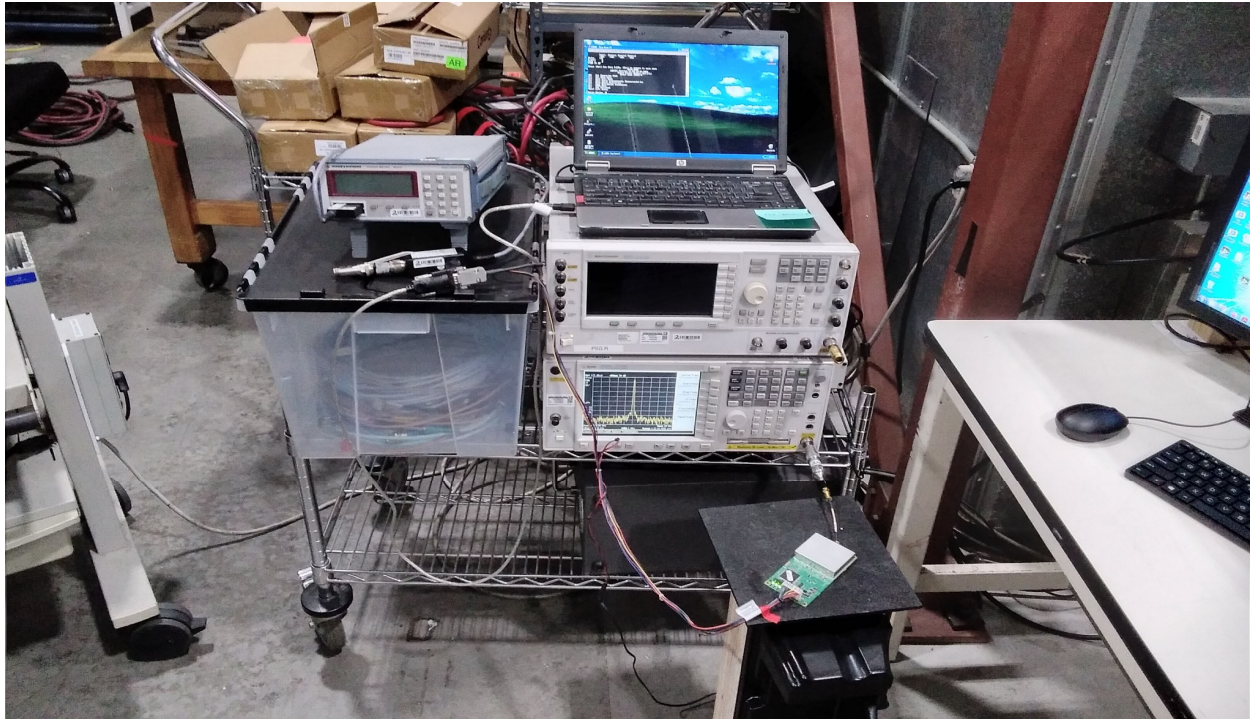
Test Configuration Photograph #3 (Antenna Conducted Emissions)
