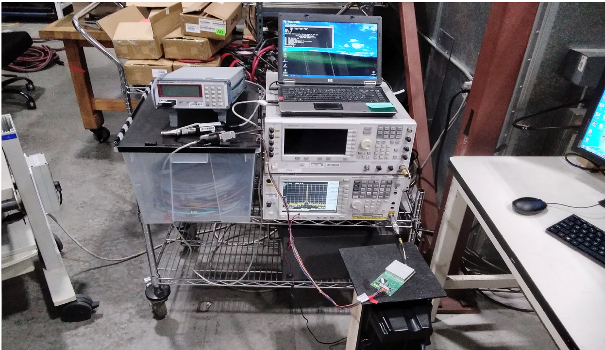
Test Configuration Photograph #1 (Conducted Emissions - RF Port)
