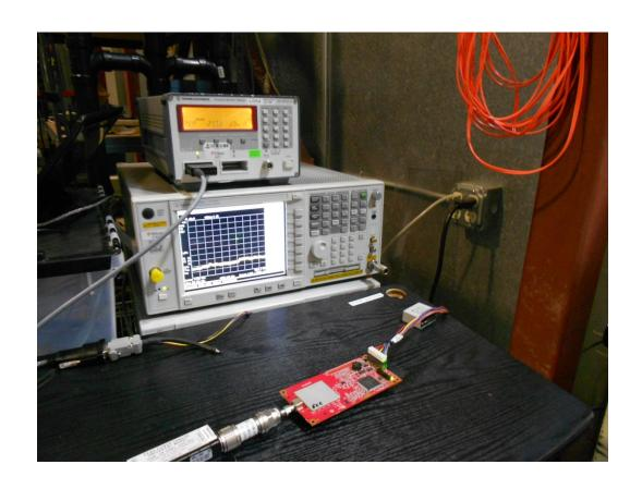
AC Power Conducted Emissions Test Configuration Photographs
