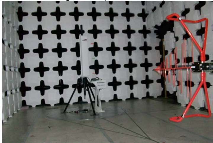
Ridge-Guide Horn Antenna (1GHz to 18GHz)
