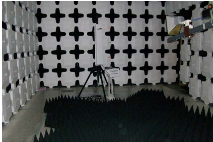
Ridge-Guide Horn Antenna (1GHz to 18GHz)
