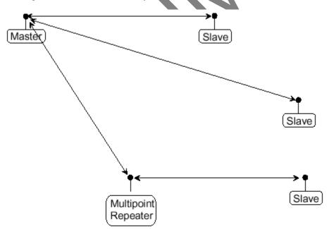
The last example is a Point-to-MultiPoint network which uses one of the sites as a Slave/Repeater. This network functions in the same manner as a standard MultiPoint network with Repeaters. However, the number of radios may be reduced with the use of the MultiPoint Slave/Repeater feature.
