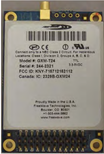
GXM-24 Top and Bottom (24-pin interface connector, 3.3-5VDC)
