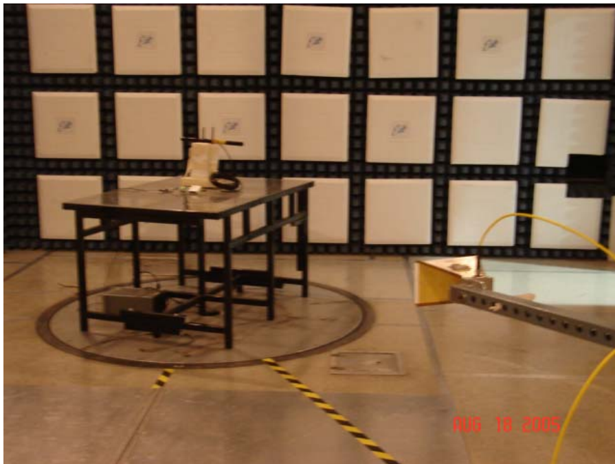
Test Setup for Radiated Emissions with the Yagi Antenna - Vertical Polarization
