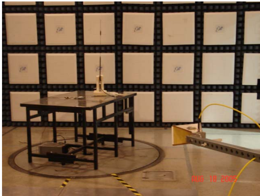
Test Setup for Radiated Emissions with the Omni Antenna - Vertical Polarization
