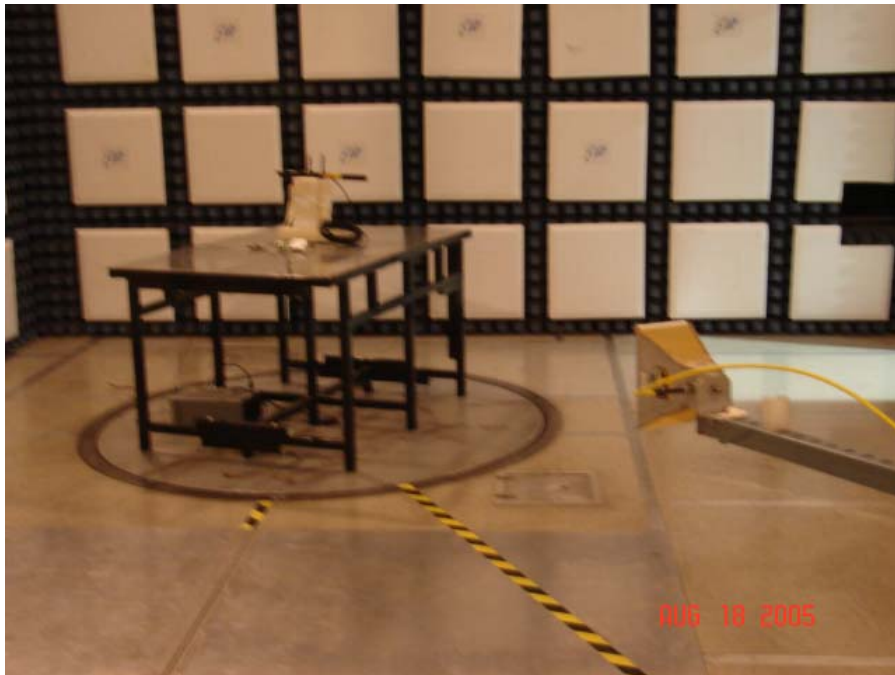
Test Setup for Radiated Emissions with the Yagi Antenna- Horizontal Polarization
