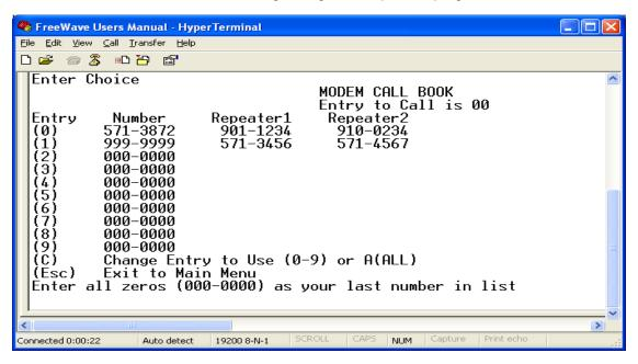
It is important that the Call Book slots (0-9) are filled sequentially starting with slot 0. When a Master is instructed to Call All, it will call all Slaves listed until it reaches the first serial number of 000-0000. If a serial number is entered after the all zero number or as a Repeater, it will not be recognized as a valid number by the Master.
