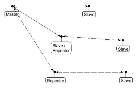
The next example depicts a standard Point-to-MultiPoint network. From the Master, any data is broadcast to all three Slaves, one of which receives it through a MultiPoint Repeater. The data is in turn sent out of the serial port of each of the three Slaves. The end device should be configured to interpret the serial message and act on it if necessary.
