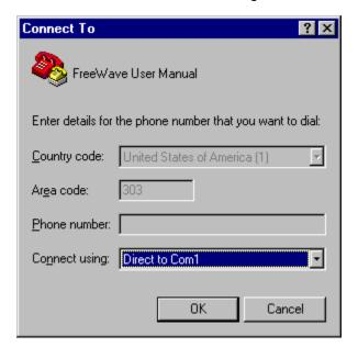
5. Select the connection type to be used from the **Connect using** drop-down menu. In most cases the connection type will be either **Direct to Com1** or **Direct to Com2**.
