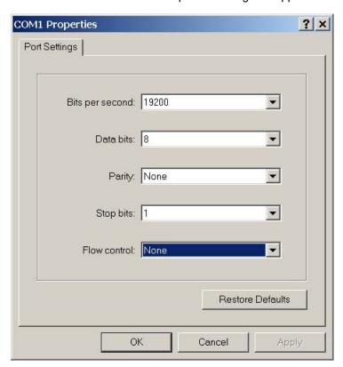
The following are the port settings which must be set for a proper connection:
