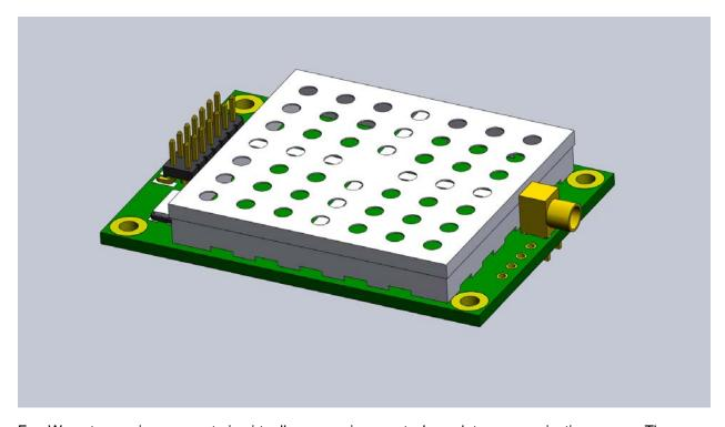
FreeWave transceivers operate in virtually any environment where data communications occur. The radios act as data transmission devices, duplicating data in either a Point-to-Point mode (one data transmitter to 1 data receiver) or Point-to-Multipoint mode (1 data transmitter to multiple data receivers).
