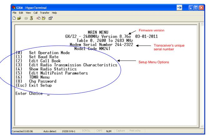
The following section describes in detail how to use all of the Setup menu options to edit the operational parameters and view the performance data.
