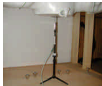
Figure 12.1 Dipole Validation Test Setup
