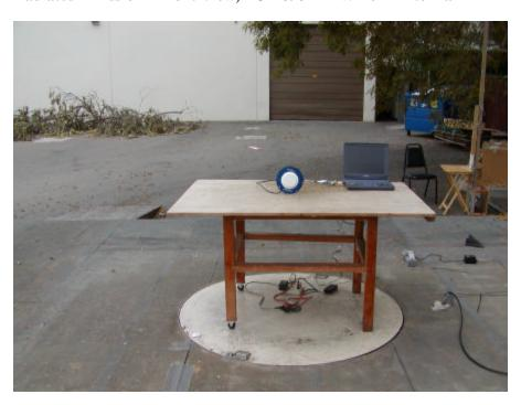
Radiated Emission - Rear View, EUT & 31717W-D/A Antenna
