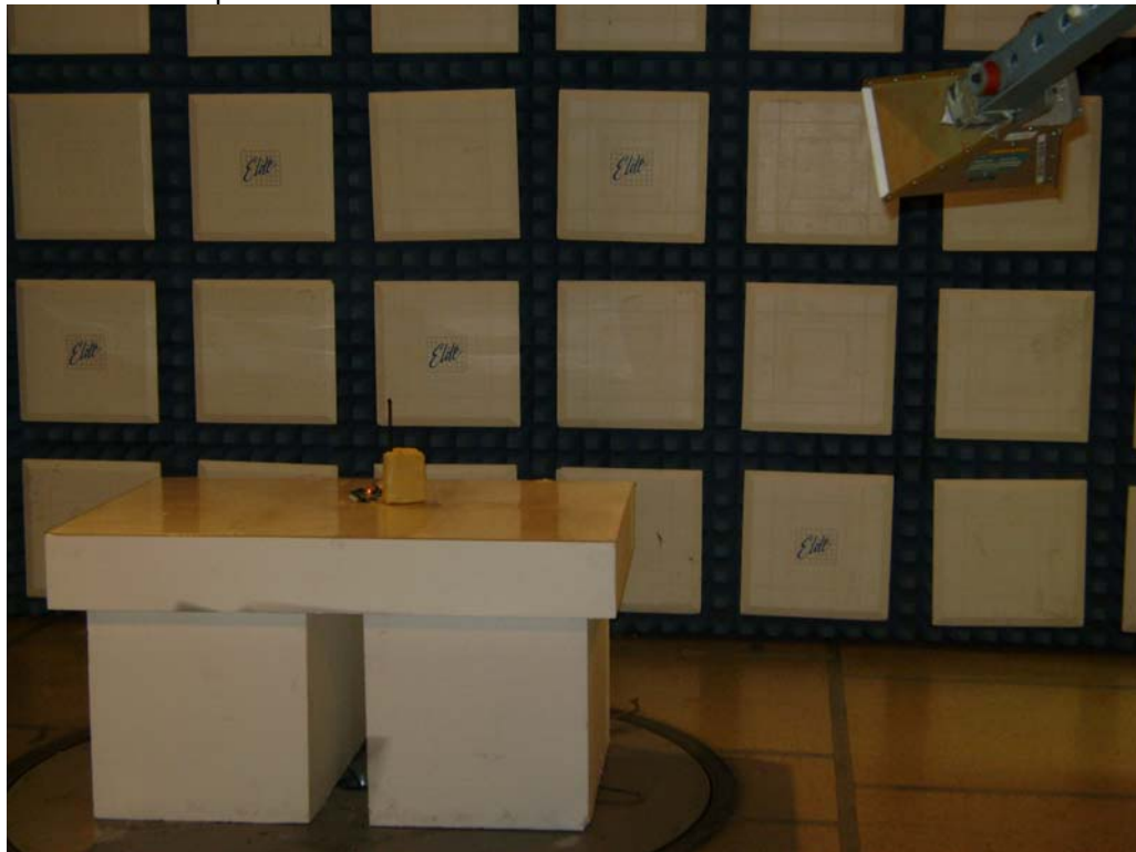
Test Set-up for Radiated Emissions Omni Antenna – Vertical Polarization
