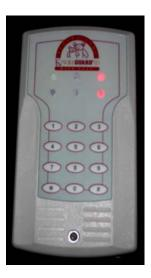
• Within a 2 foot range of the exit panel antenna, press and hold the red button on the Escort Pendant for 3 continuous seconds until the panel beeps and the top center light flashes red.
