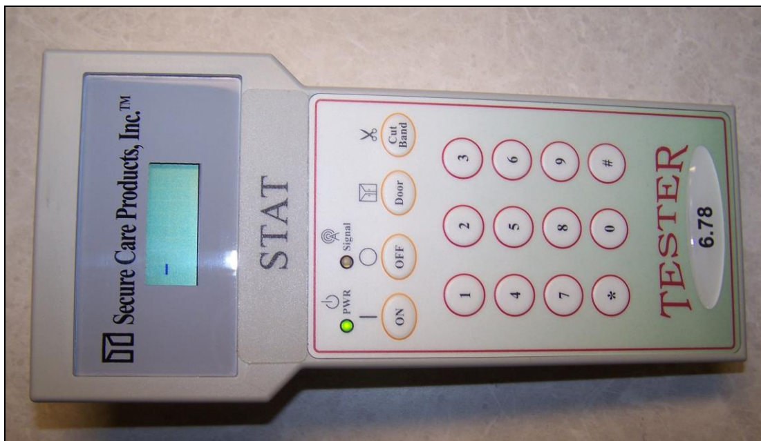
Photograph 1. Secure Care Products, 433.92 MHz System Tester.
