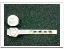
3. Test the Transmitter using the Tester to verify the ID code as shown below.
