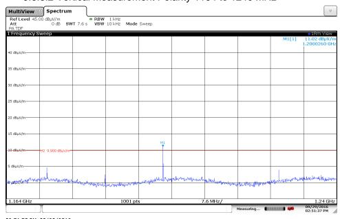
Note: Narrow band emission @ 1.2000 GHz fails under 15.209 limit
