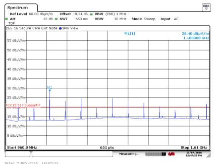
6.5.4. 960 MHz to 1610 MHz Vertical at 1 Meter (UWB Disabled)
