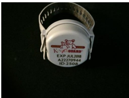
Figure 2-5 - Transmitter with strap inserted. The grey to the inside.
