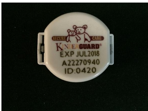
Figure 2-1 SC-40 STAT ID 90° Cutband Transmitter
