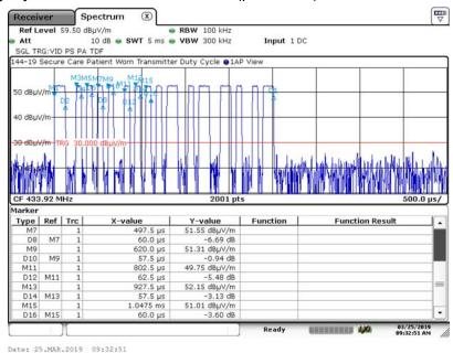
7.8.1c Duty Cycle for the Device as Tested (plot 3 of 4)
