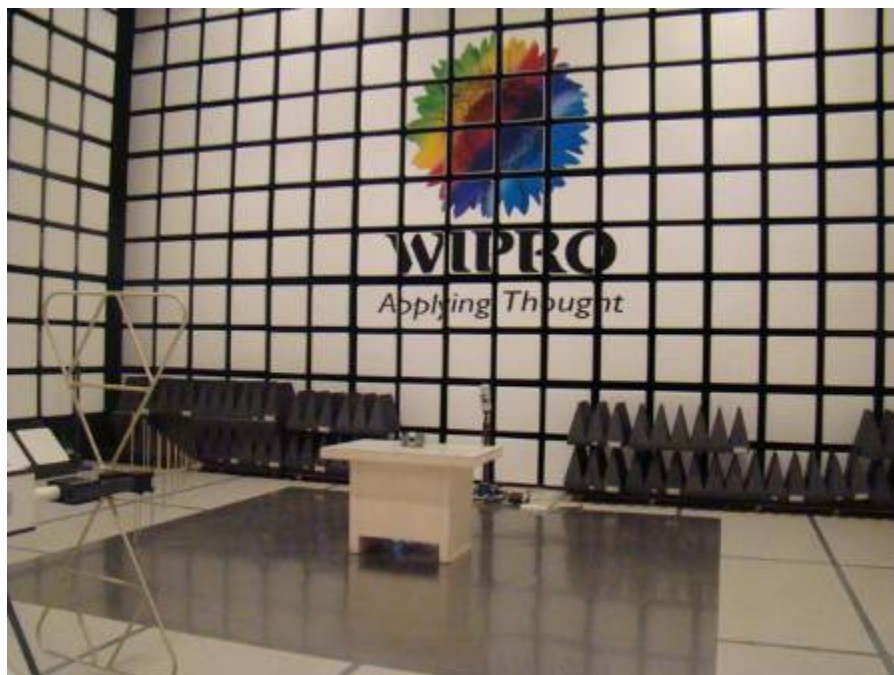
Figure 147: Test setup for Radiated Emission (Vertical polarization) – 30MHz to 1GHz
