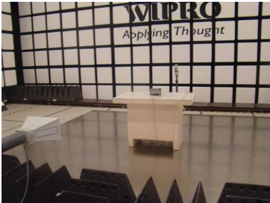
Figure 150: Test setup for Radiated Emission (Vertical polarization) – Above 1GHz
