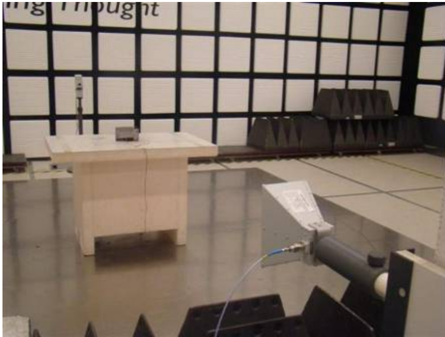
Figure 149: Test setup for Radiated Emission (Horizontal polarization) – Above 1GHz
