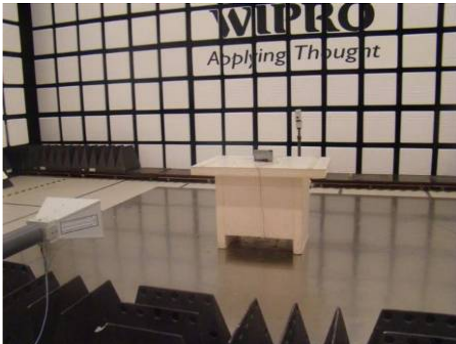
Figure 64: Test setup for Radiated Emission (Vertical polarization) – Above 1GHz
