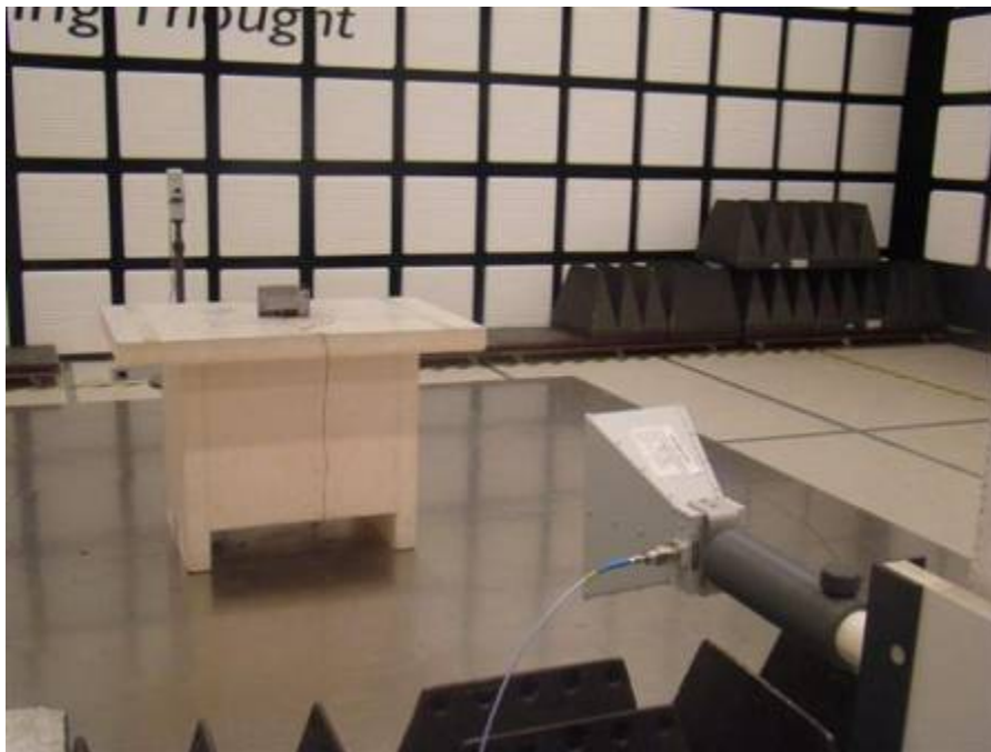
Figure 63: Test setup for Radiated Emission (Horizontal polarization) – Above 1GHz
