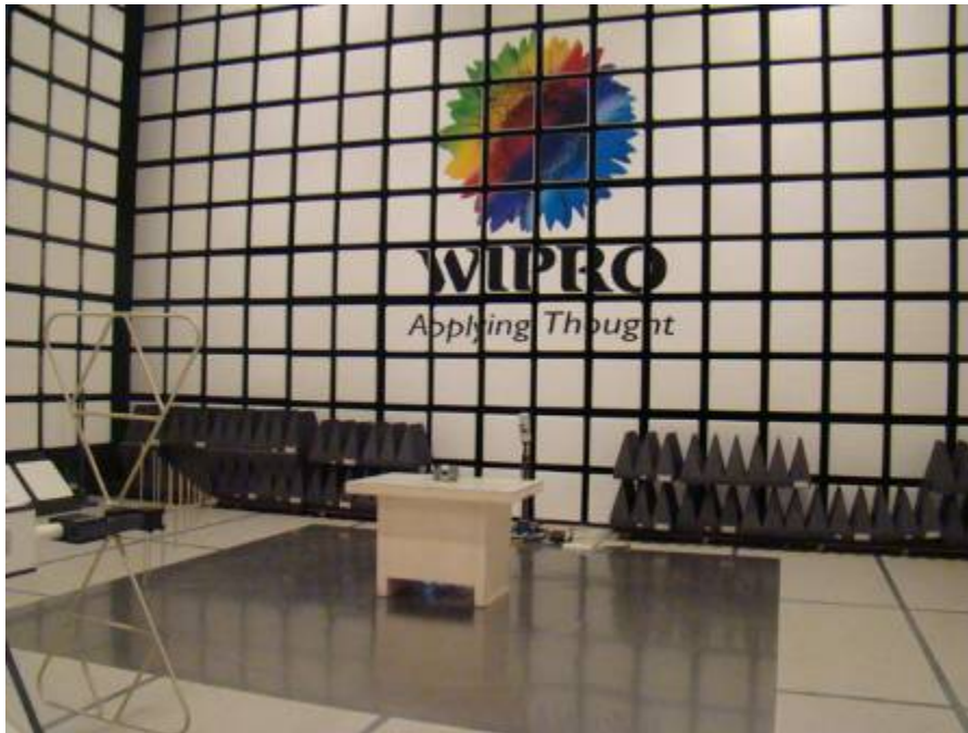
Figure 61: Test setup for Radiated Emission (Vertical polarization) – 30MHz to 1GHz
