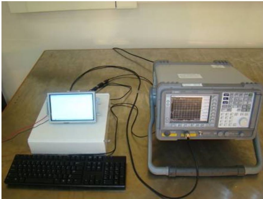
Figure 65: Test setup for Conducted measurements
